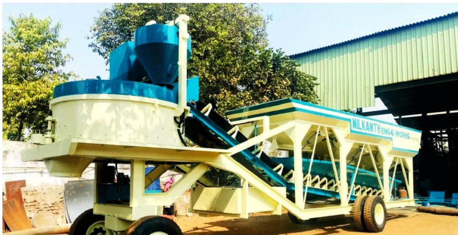
Fig: Mobile Concrete Plant
