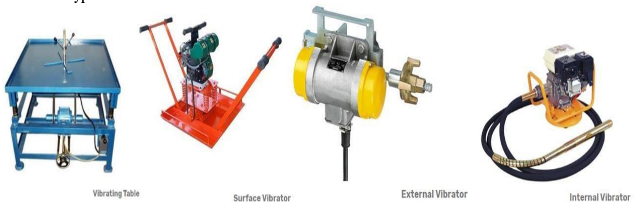
Fig: Concrete Vibrators
